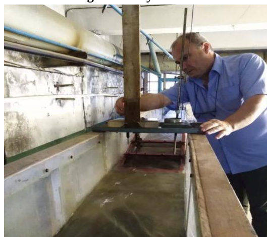
Fig. 9. Debris flow regulation elastic barrage during the laboratory tests
